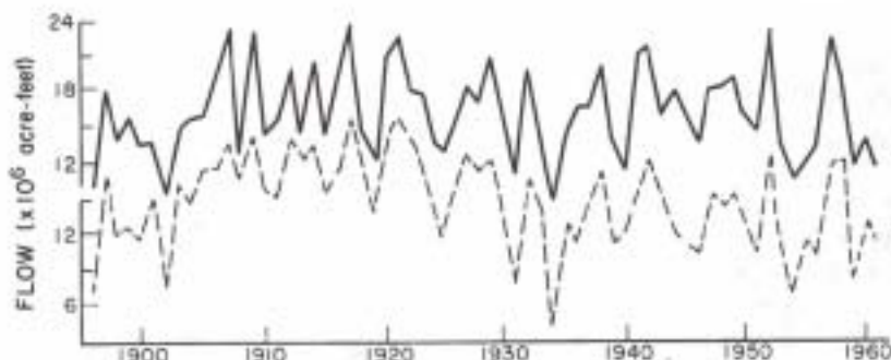
FIGURE 10.28 Runoff in the Upper Colorado River Basin. Reconstructed values (—) are based on tree-ring width variations in trees on 17 sites in the basin. Actual data, measured at Lee Ferry, Arizona, are shown for comparison (---). Based on this calibration period, an equation relating the two data sets was developed and used to reconstruct the flow of the river back to 1564 (Fig. 10.29) (Stockton, 1975).
